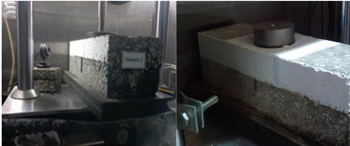
Fig. 3. The UTM225 test device used for testing.
