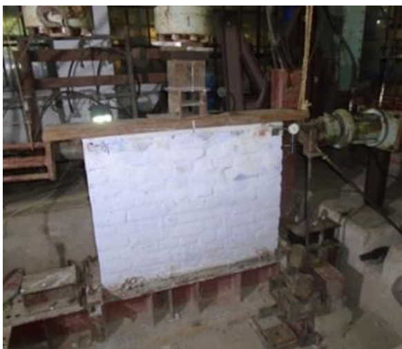
Fig. 4. Experimental setup before starting the test.
