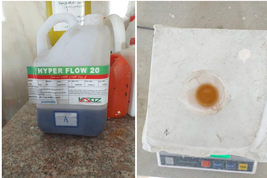
Fig. 4. The color and type of the Polycarboxylate-Lignosulfonate Superplasticizer used in the study.
