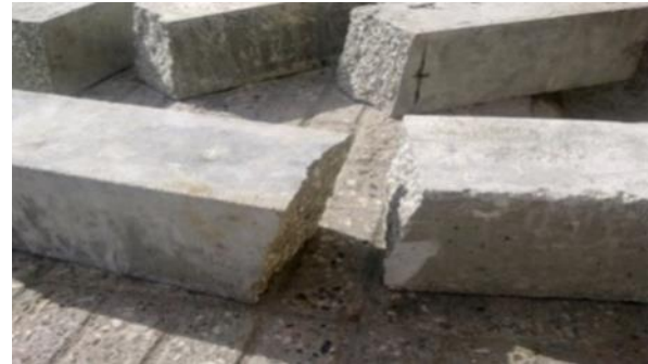
Fig. 20. A broken specimen in splitting tensile strength test.
