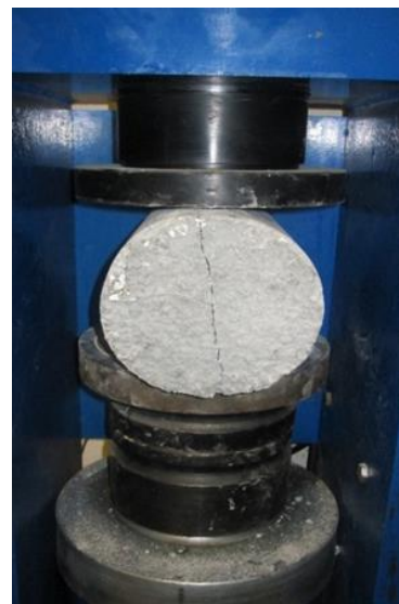
Fig. 10. Splitting tensile Strength test.
