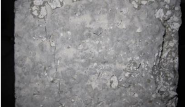
Fig. 14. A broken specimen in compressive strength test.
