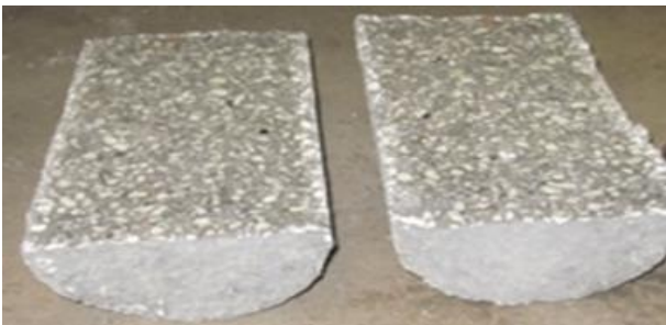
Fig. 17. A broken specimen in splitting tensile strength test.
