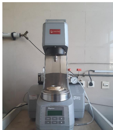
Fig. 2. A view of the DSR test apparatus.
