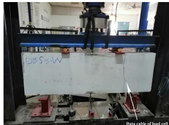
Fig. 6. Experimental Setup for Load Testing of Lightweight Reinforced Concrete Deep Beams.
