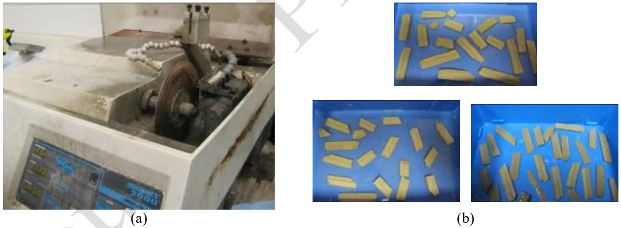
Fig. 6. High precision saw (a) and single fiber specimens cut ready for testing (b).
