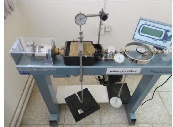
Fig. 4. Direct shear apparatus used in experimental program
