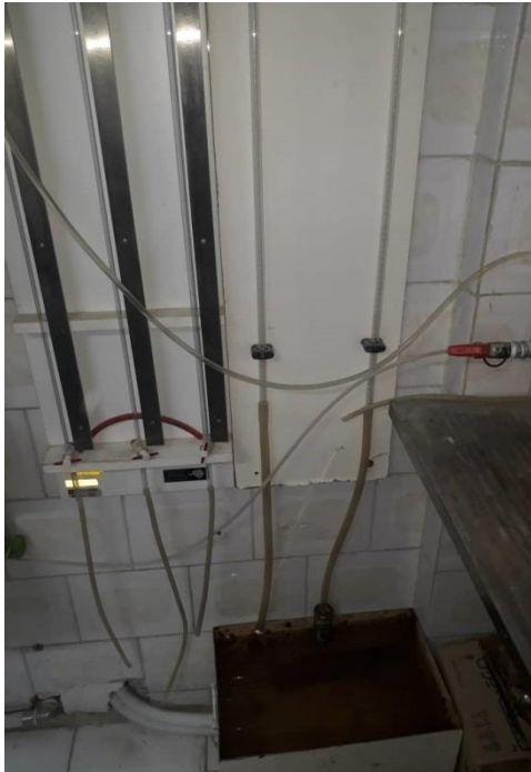
Fig. 5. Permeability apparatus used in experimental program.
