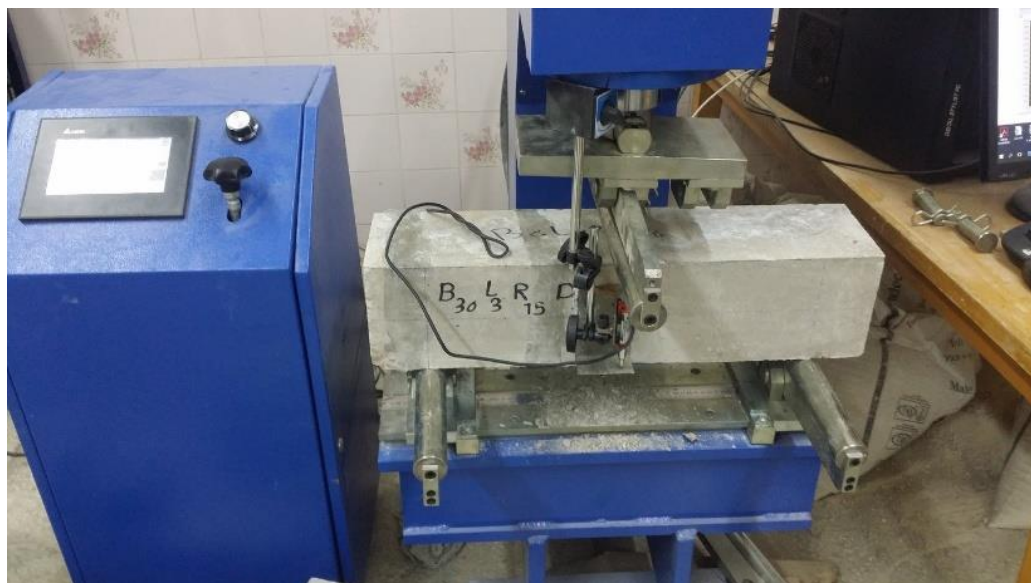
Fig. 4. Three-point bending jack machine used in the research.
