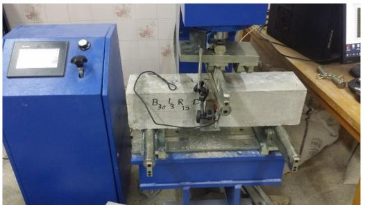
Fig. 4. Three-point bending jack machine used in the research.
