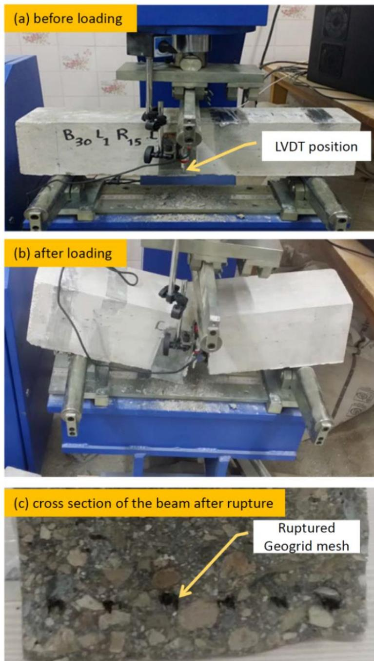
Fig. 6. A detailed sample of the tested specimen and its cross-section. 4. Results and discussion.
