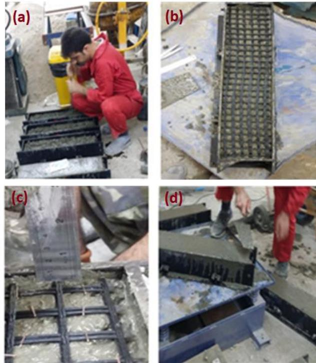
**Fig. 3.** (a) Casting the first part of fresh concrete; (b) Placing the GFGM; (c) Controlling the placement of GFGM (d) Casting the second part of the concrete and compacting the specimen by the vibration table.
