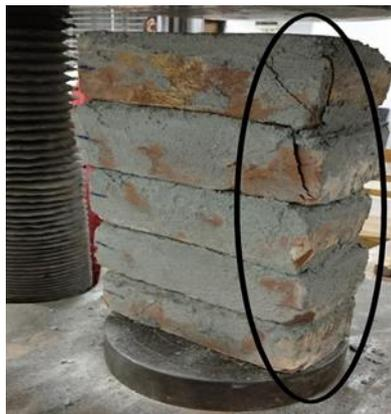
Failure pattern for Masonry Prism; c/s=1:3
