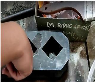
**Fig. 6.** Lubrication of Mold.
