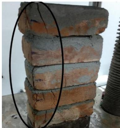
Failure pattern for Masonry Prism; c/s=1:4
