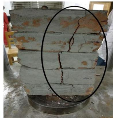
Failure pattern for Masonry Prism; c/s=1:5
