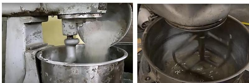
**Fig. 5.** Mixing of Mortar using a mixer machine in the laboratory.
