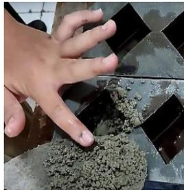
**Fig. 7.** Placement of mortar in mold.
