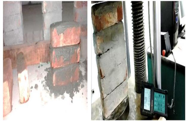
Fig. 14. Prism Test using Universal Testing Machine (UTM) in Laboratory.
