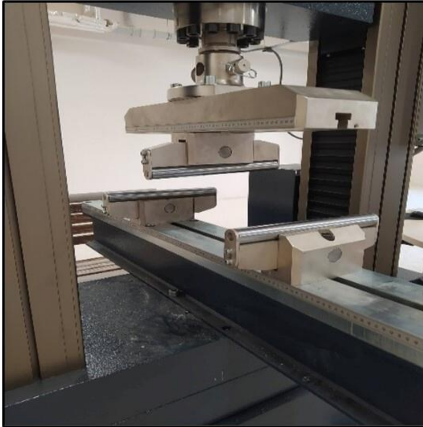
Fig. 5. Three-Point Bending Test Apparatus Located in the Construction Laboratory of the Civil Engineering Department at Ankara University.
