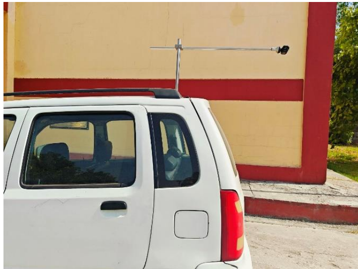
Fig. 4. The mounting stand is fixed on the top of the vehicle.
