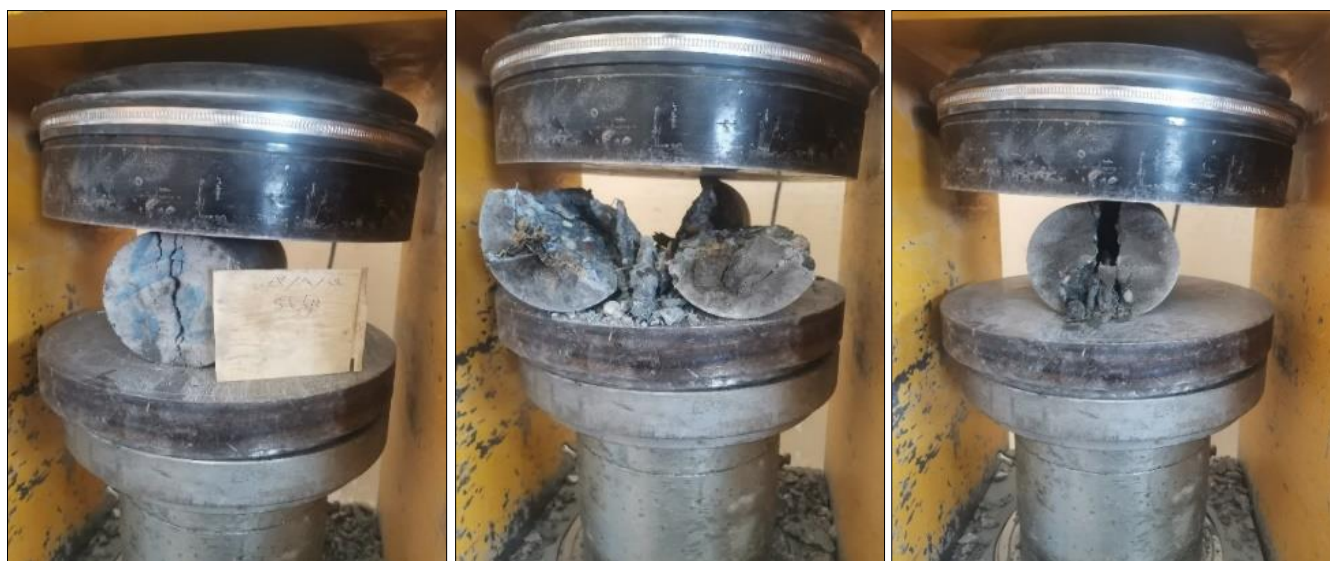
Fig. 9. Photo of Split Tensile Strength Test.
