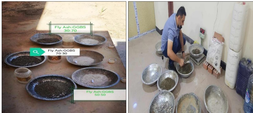
Fig. 5. Mixing of Geopolymer concrete.
