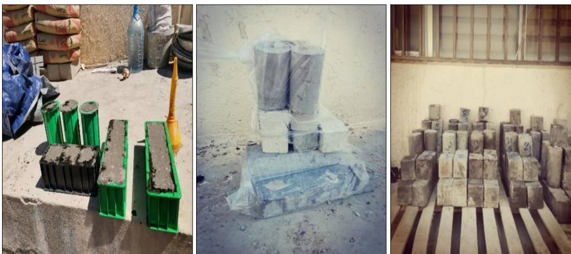
Fig. 6. Casting and curing of specimens.
