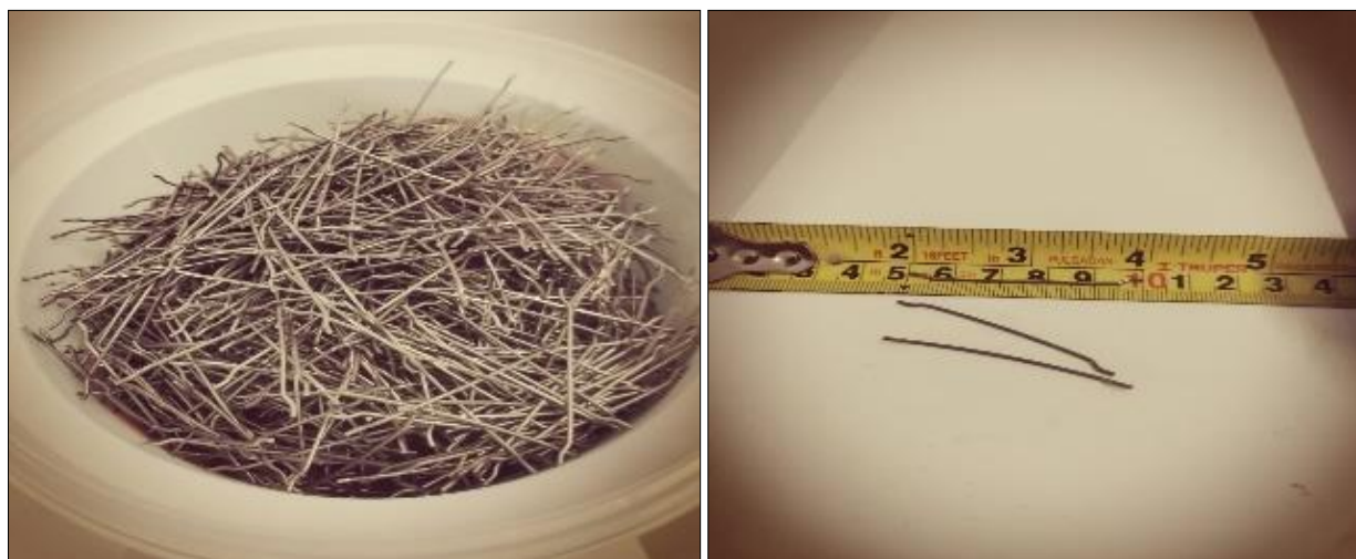
Fig. 2. Hook-end Steel Fibbers.
