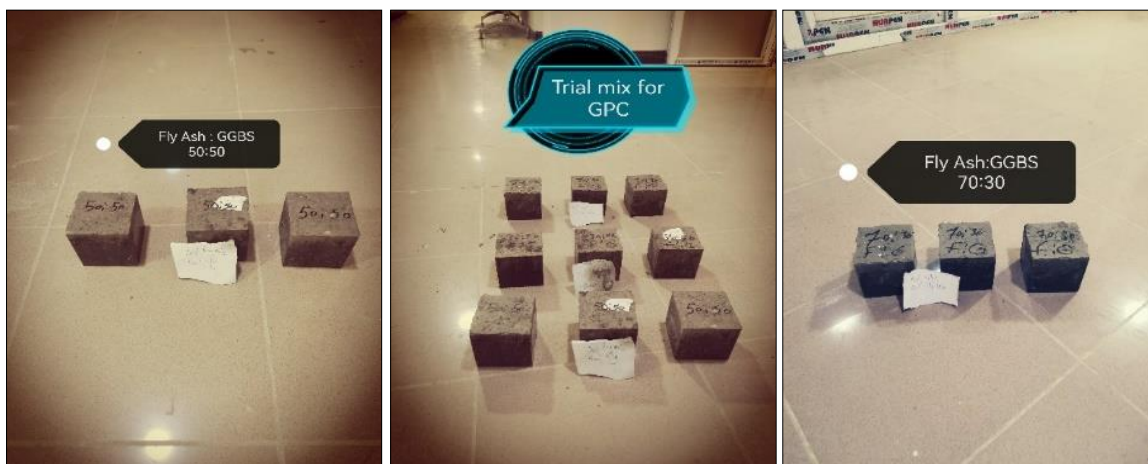
Fig. 3. Trail mix cubes for geopolymers mix.
