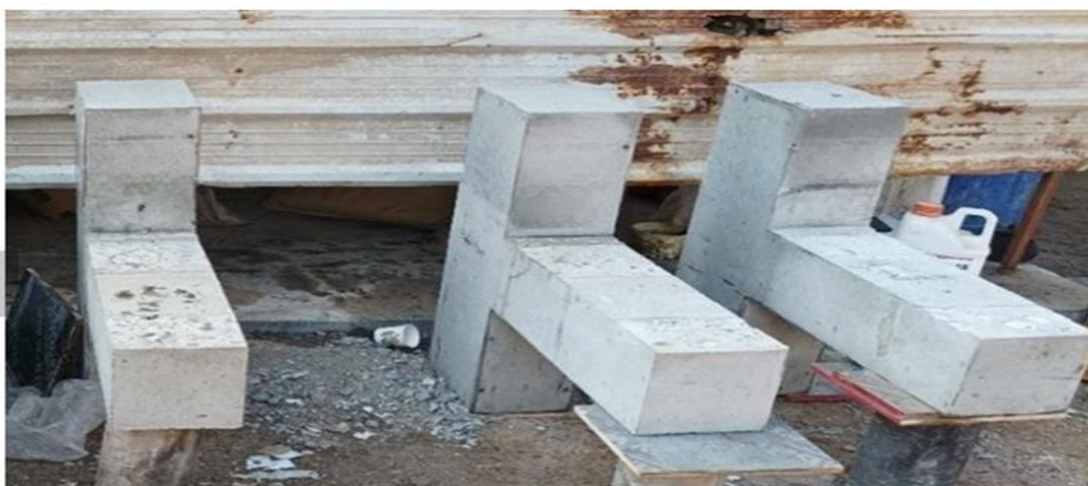
Fig. 2. Beam-column joints specimens.
