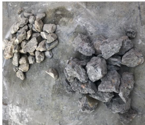
Fig. 9. A real picture of recycled aggregates versus natural aggregate.
