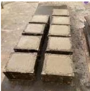
(a) Mortar cubes for compression test.
