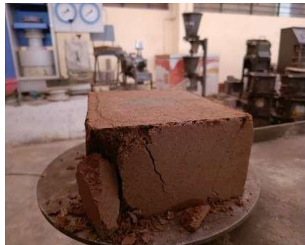
(b) Failure pattern of the tested specimen.
