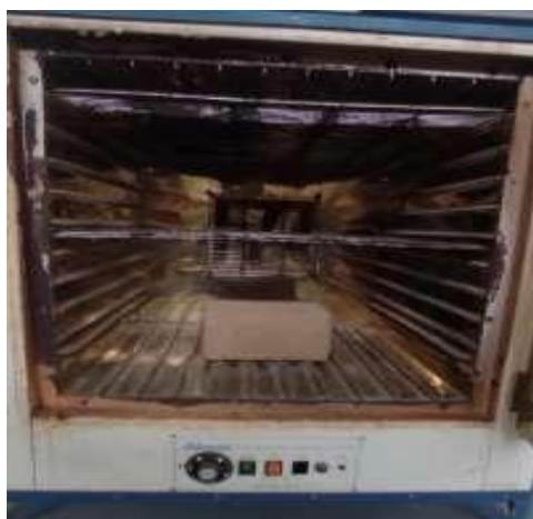
(a): Oven drying of block.
