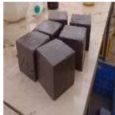
(b) Demoulded cubes of size 70.7 mm.
