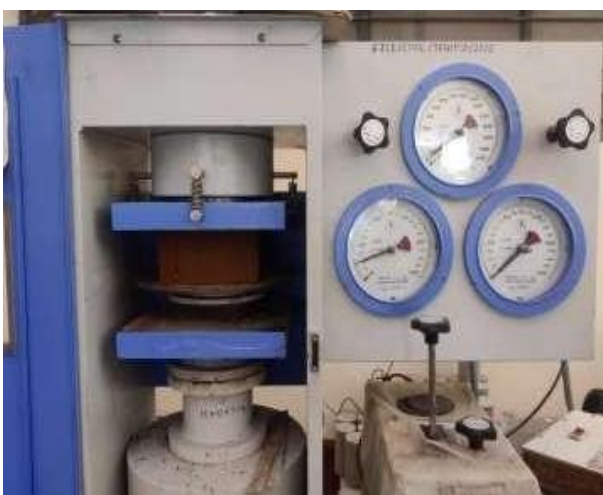
(a) Block placed in compression testing machine.
