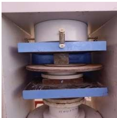
(c) Cube placed in test setup.
