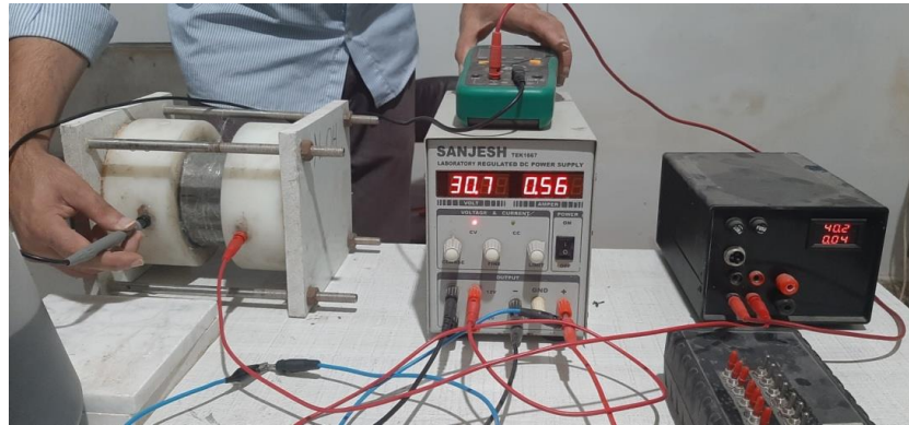
Fig. 7. RCP test setup.
