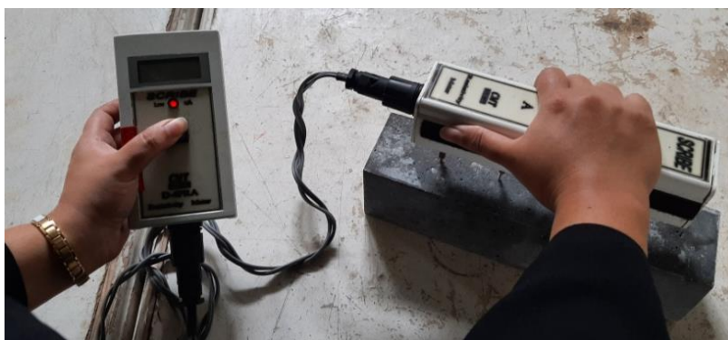
Fig. 6. 4-pin Wenner probe for electrical resistance of concrete.
