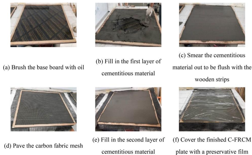
Fig. 6. Process of prefabricated C-FRCM plate. Reproduced with permission from Feng et al. (2022) [23].
