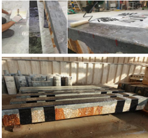
Fig. 4. Process for applying CFRP. Adapted from Kharmah et al. (2022) [27].
