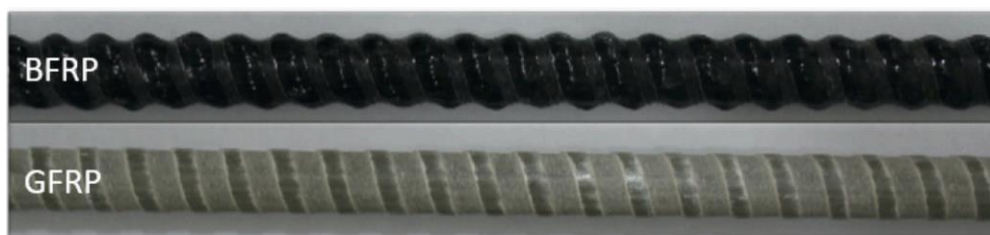
Fig. 1. NSM–BFRP and NSM–GFRP bars were employed to reinforce and improve the structural integrity of the slabs. Adapted from Aljidda et al., (2023) [14].
